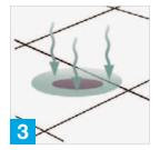
Scrub surfaces with a rotary scrubber to release cement & salt residues.
