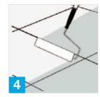
When dry and free of residues apply a final coat of protector making sure to cover the joints as well.
