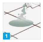
Ensure surface to be treated is clean and as dry as possible before pouring the sealer onto the surface.
