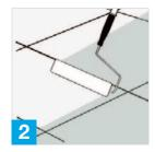
Spread out evenly using a sealant applicator pad, broad paint brush or foam roller. Repeat after 30 minutes. Leave to dry for 1 hour.
