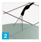
Wet the surface with the solution and leave for 10-15 minutes.
