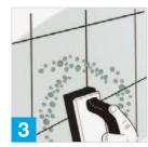
Add a little water and gently scrub surfaces with a black pad to release any loosened matter from the surface.
