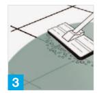
Add a little water and gently scrub surfaces with a black pad to release the loosened matter from the surface.
