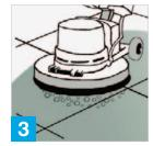
Releasing water from the on board tank and scrub surfaces and grout joints to release the dirt and grime.
