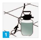
Dilute solution 1:1 with warm water and fill a light pressure sprayer.
