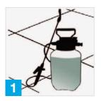
Dilute solution 1:1 with cool water. Mask and protect areas not to be cleaned.
