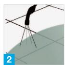
Set the pressure between 0.5 and 1 bar. Apply an even layer to the surface.
